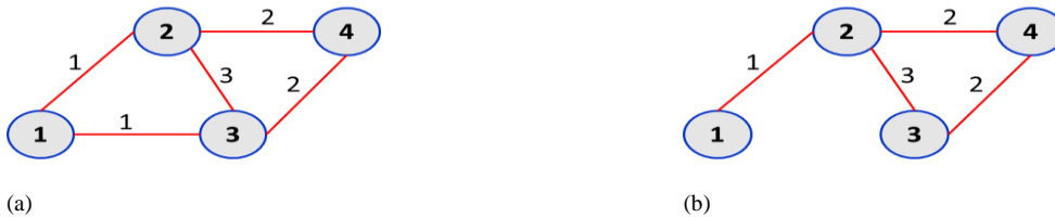
Figure 1: Map corresponding to a country with four (04) cities which are represented as nodes. The edges correspond to the length of the highway between any two cities.
